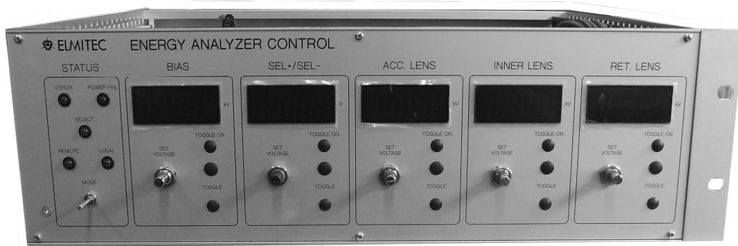
Front Plate of ELMITEC Analyzer Control
