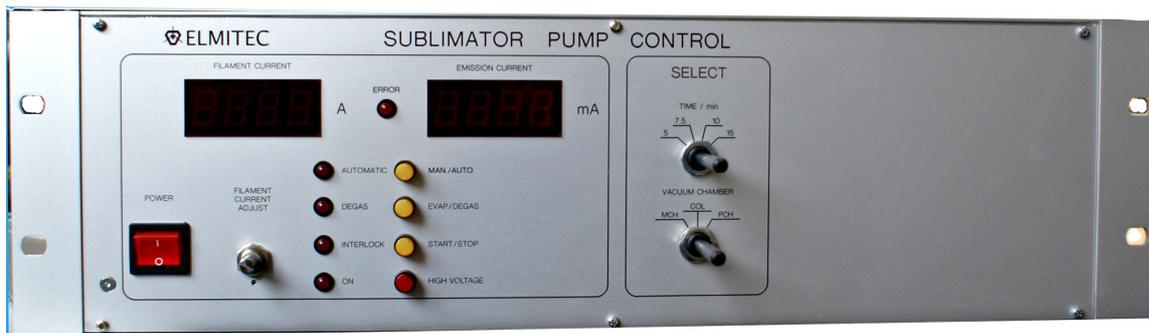
Frontside of ELMITEC Ti Sublimation PUMP Supply
