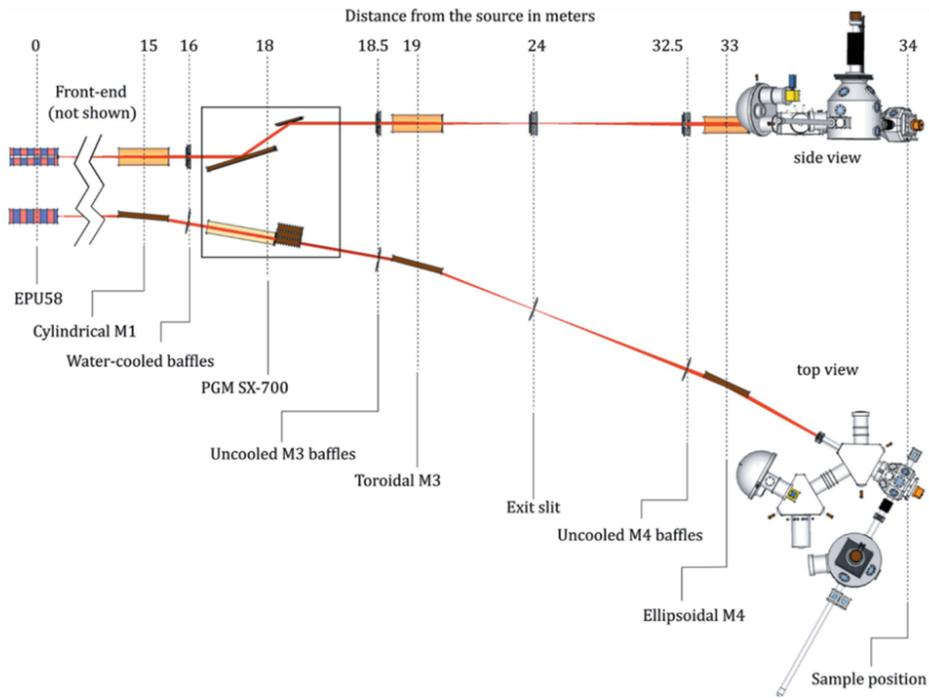
**Figure 2.** Schematic of the optical layout of the MAXPEEM beamline.
