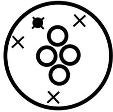
There is only one direction that the plug can be pushed to the end and be fixed.
