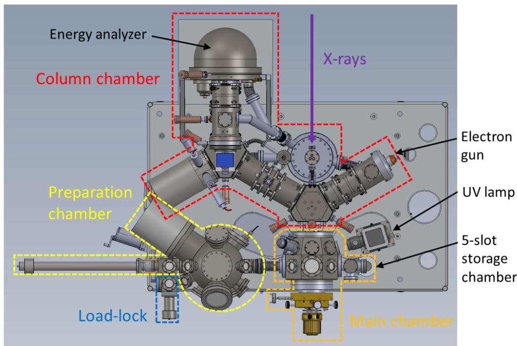
**Figure 4.** Top view schematic of the MAXPEEM spectro-microscopy endstation, showing key vacuum chambers and the three (photo-)excitation sources: (i) beamline, (ii) UV lamp and (iii) electron gun.
