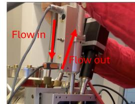
(Valve 2) This direction for gas flowing to main chamber.
