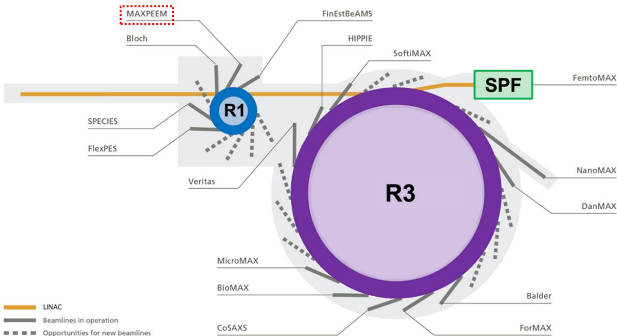
**Figure 1.** Schematic of MAX IV, showing the three major components: (i) linear accelerator (LINAC), (ii) 1.5 GeV electron storage ring (R1), and (iii) the 3.0 GeV electron storage ring (R3).
