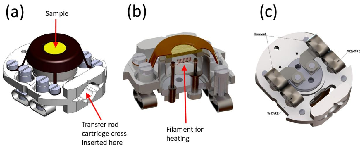
Figure 1. CAD drawings of the Elmitec sample holder, showing (a) the fully assembled sample holder with sample, (b) a cut-away of the sample holder exposing the heating filament, and (c) the underside of the sample holder.
