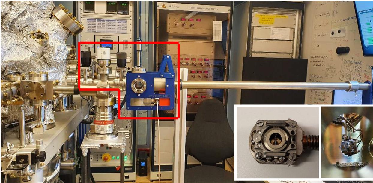
Figure 1. Photo of the Ferrovac UHV suitcase connected to the prep chamber. The inset shows the Elmitec-Omicron adaptor,
